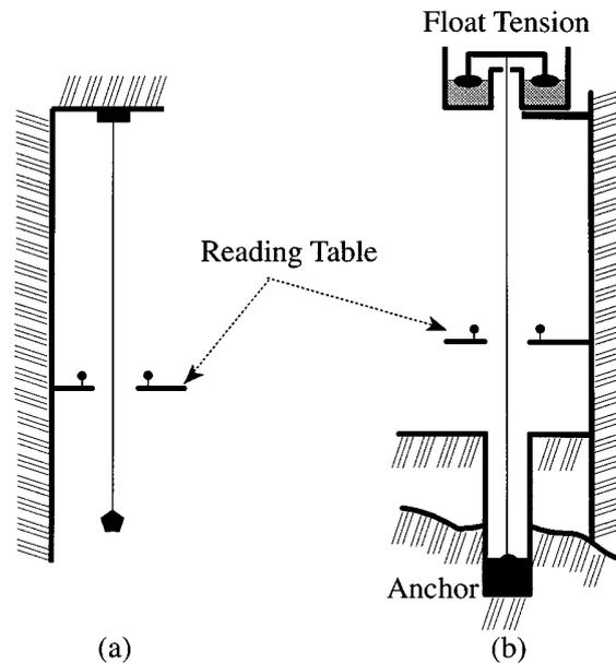
FIGURE 15.4 Inclination measurements with plumb lines. (a) suspended pendulum; (b) inverted pendulum.
