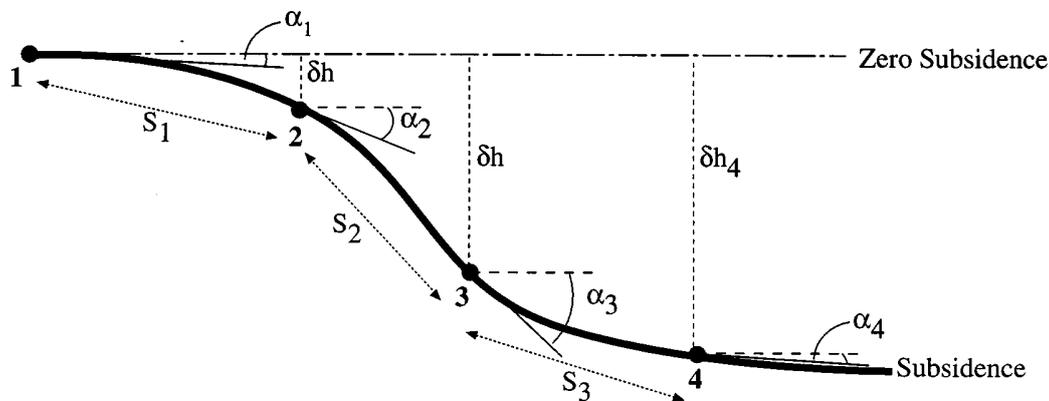
FIGURE 15.1 Ground subsidence derived from tilt measurements.
