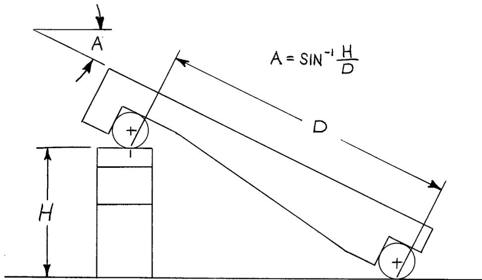
**FIGURE 14.2** Sine bar. A sine bar is used in conjunction with precision gage blocks that are placed under one of the cylindrical rods, raising that end a distance,  $H$ , equal to the sine of the desired angle times the distance,  $D$ , between the two rods.
