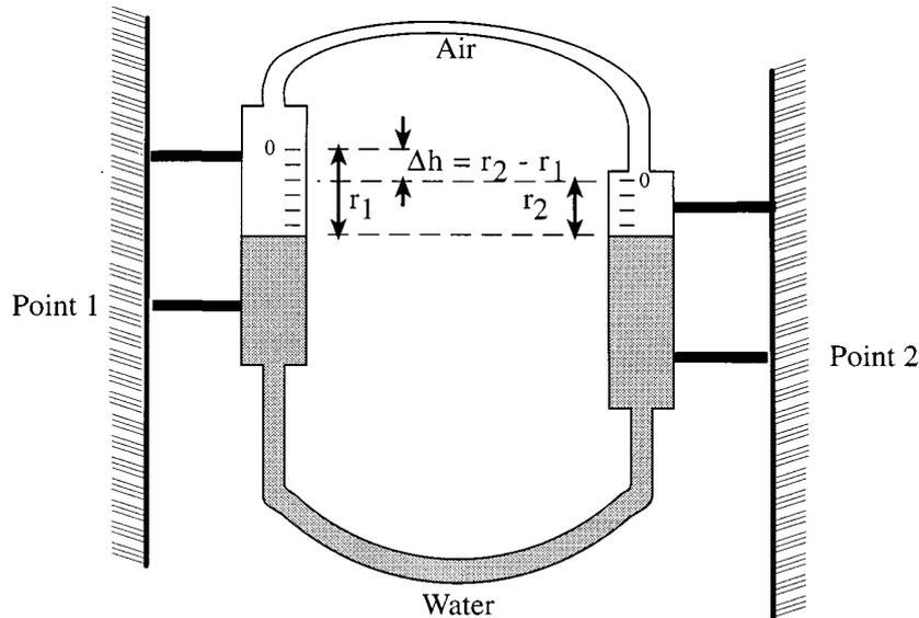
FIGURE 15.3 Hydrostatic leveling ( $\Delta h_{12} = r_2 - r_1$ ).
