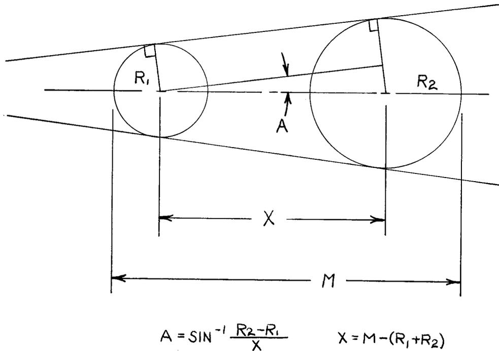
**FIGURE 14.3** Measuring tapers. Two balls (for holes) or gage pins (for slots) should be selected to fit the hole size to be measured. The distance between the balls or pins should be as large as possible to allow for the best accuracy of measurement. The position of the balls can be determined and the equations shown in this figure applied to determine the angle of the taper.
